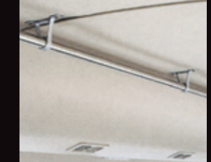
Ceiling grab rail For easier standing and moving
