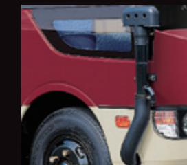
Snorkel air intake Protects engine from dust
